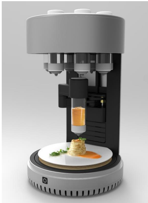
Figure 6. Extrusion printing for the food industry. Source: Grup de recerca de la Universitat de Columbia - https://www.creativemachineslab.com/digital-food.html , CC BY-SA 4.0, https://commons.wikimedia.org/w/index.php?curid=84202502
