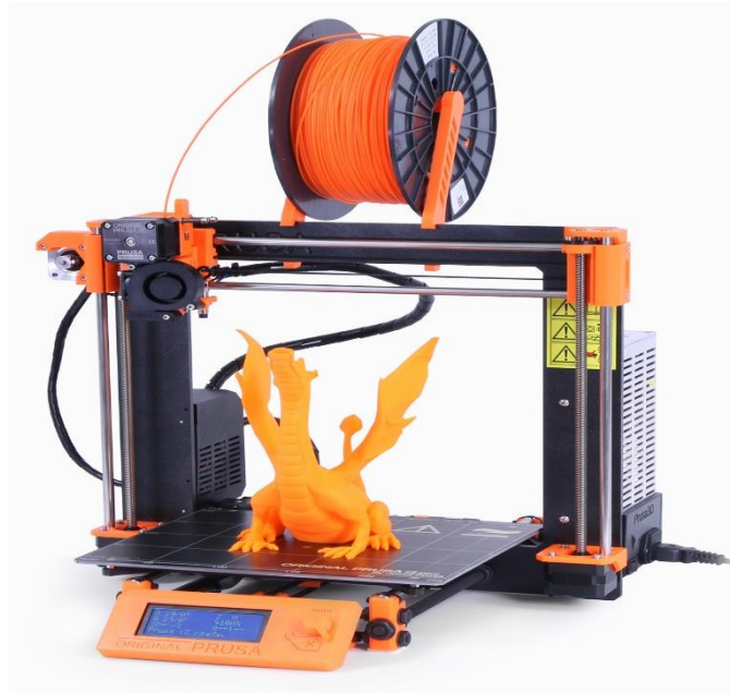
Figure 5. PRUSA i3 MK2 FDM printer (Prusa Research, Prague, Czech Republic) with spool and a completed object. Image source: Wikimedia Commons, http://reprap.org/wiki/File:Prusai3-MK2.jpg .
