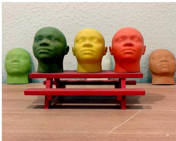
Figure 7. Rapid prototypes manufactured by powder-based 3D printing. Source: S Zillayali, CC BY-SA 3.0 < https://creativecommons.org/licenses/by-sa/3.0/ >, via Wikimedia Commons
